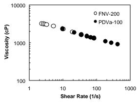
Viscosity measured by using the portable/ disposable viscometer (PDVa-100) compared to the data measured by the falling needle viscometer (FNV-200) for ointment at 25°C
