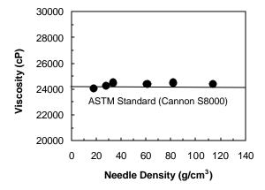
Viscosity measured by using the portable/ disposable viscometer compared to the data known of ASTM standard (Cannon S 8000) at 25°C
